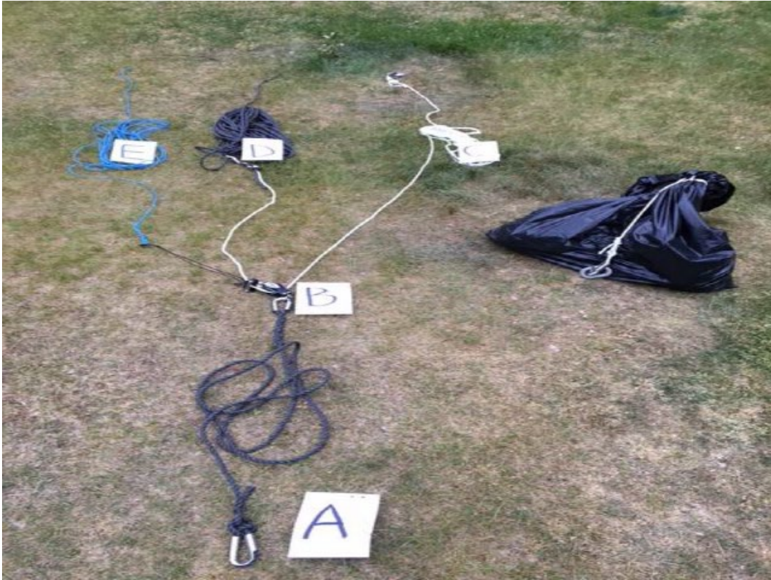
Figure 8: Photo of one of the anchor rope units.
