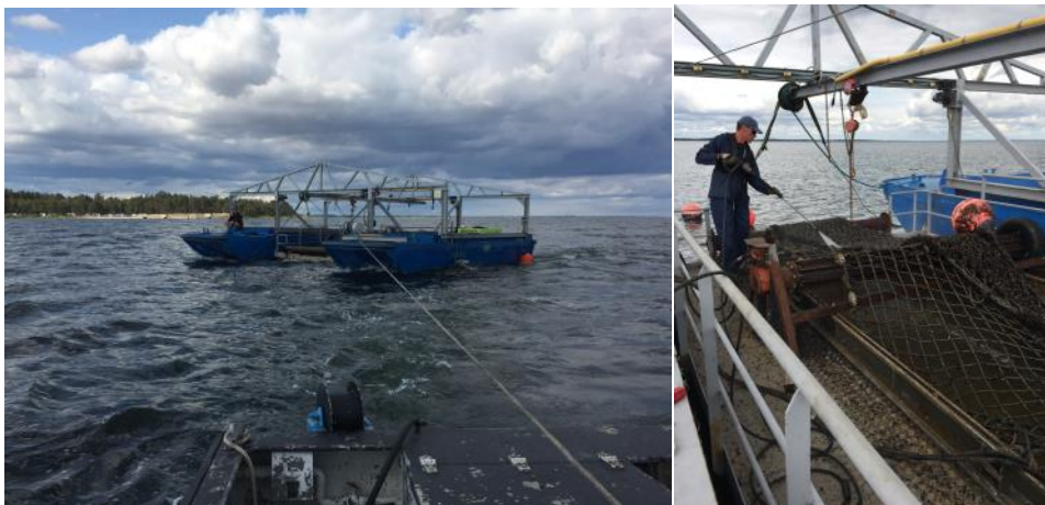
Figure 14. "Plan B" harvester. This method works for net farms that have floats and not PP-pipes for flotation.
