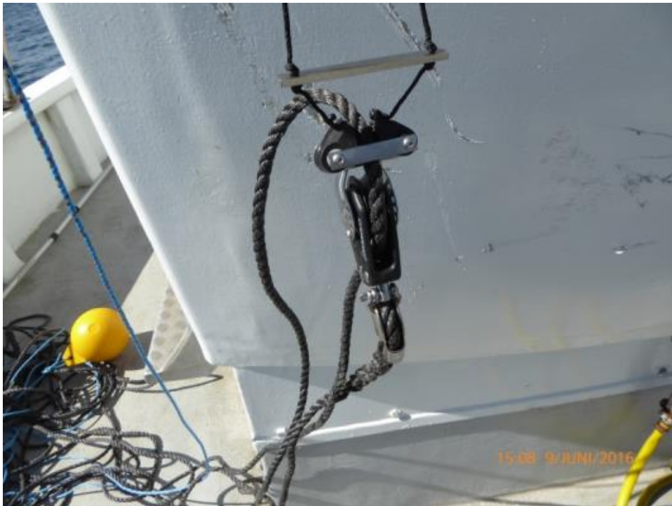
Fig 9: Close-up of an anchor- block (B in Fig. 8)
