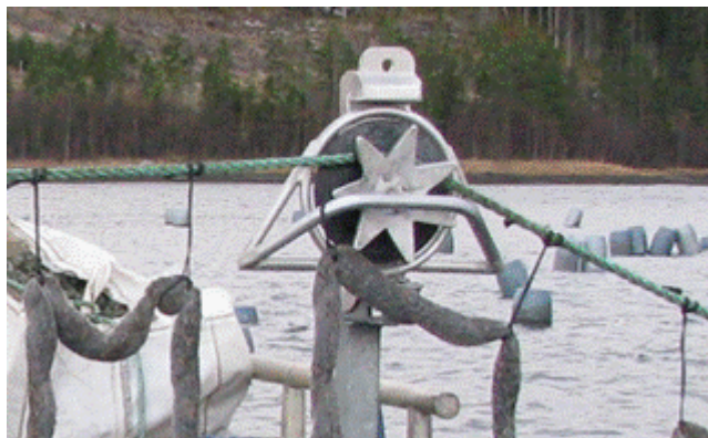
Figure 24 Mainline rolling through the starwheel
