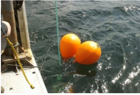
Figure 26 Float of 40 litres
