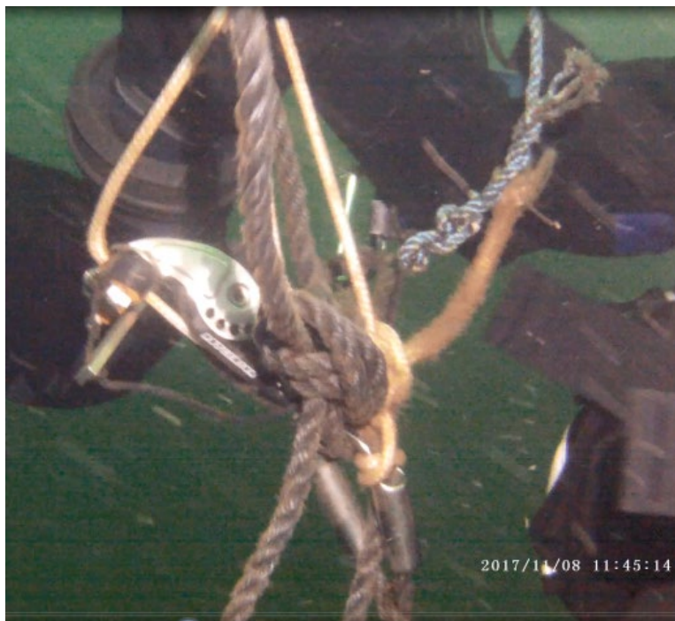
Figure 10. Block by-passed by a knot from the anchor rope (Fig. 8A) and anchor line (C) to relieve the slithering breaks.
